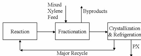
Figure 1. Simplified para-Xylene Process Flow Diagram
