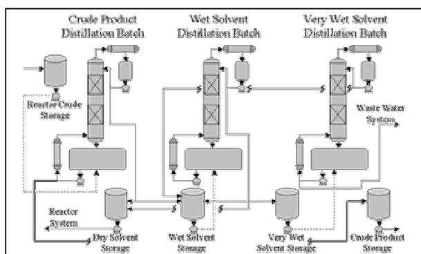
Figure 1. One Column, Three Distillations.
