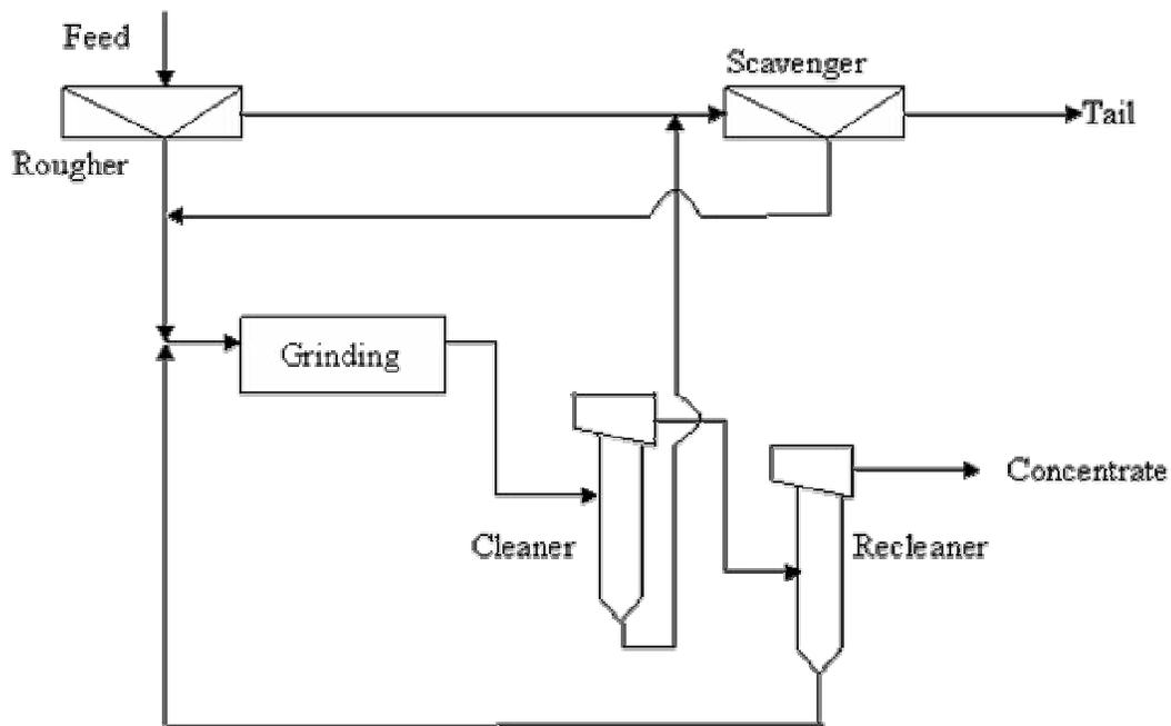
Figure 3. Optimized flowsheet for copper concentrate plant.
