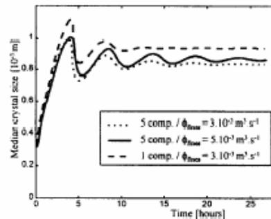
Figure 9. Results of modeling start-up of 1.1  $\text{m}^3$  DTB crystallizer with a 5 compartment cell model at two values of fines flow and an MSMR (1 compartment) model. Bermingham et al. (1998).
