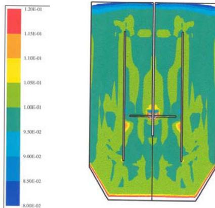
Figure 7: Prediction of particle distribution in a tank with draft tube by interpenetrating continua model. Particles: average 10 vol% 128  $\mu\text{m}$  glass spheres in water, agitator: pitched blade, 500 rpm. From Green et al. (1998).
