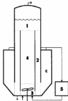
Figure 8. Identification of zones for cell model of 1.1  $\text{m}^3$  DTB crystallizer with fines destruction. Bermingham, et al. (1998).
