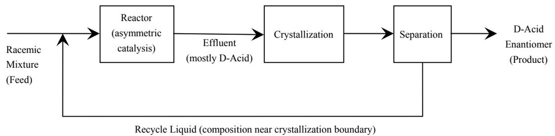
Figure 11. Flowsheet for coupling asymmetric catalysis with crystallization to produce high purity D-mandelic acid.
