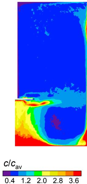
*Figure 6. Solids distribution predicted by LES & particle tracking. Rushton turbine in baffled tank, left edge of figure is tank centerline. Slice is taken midway between baffles. From Derksen (2003).*
