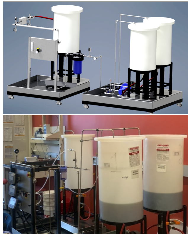
Figure 4: Pilot Plant CAD Design (Top) and Fabricated Pilot Plant Design at the Laboratory (Bottom)
