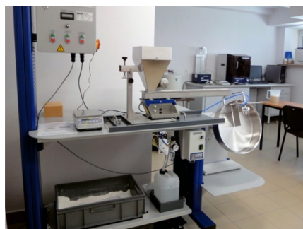
Figure 1: (Left) Experimental pan granulation setup. (Right) Schematic representation of pan granulation process
