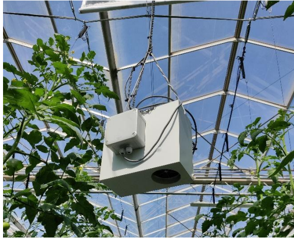
Figure 1: Temperature and relative humidity monitoring sensor.
