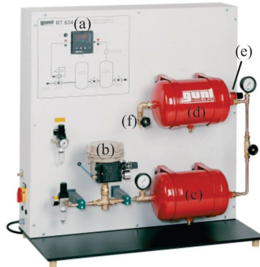
Figure 1: Pressure control demonstration unit RT-634 (Source: GUNT GmbH).
