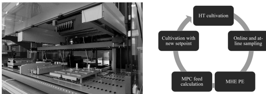
Figure 1: The high-throughput robotic facility (left) and the iterative workflow of the cultivation
