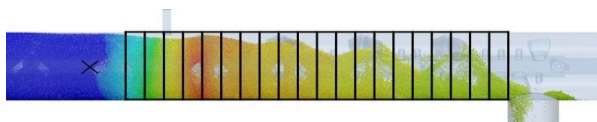
Figure 7. A model division into coloured regions as per degree for mixing analysis
