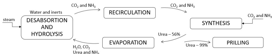
Figure 1: Simplified block diagram for the urea production process.
