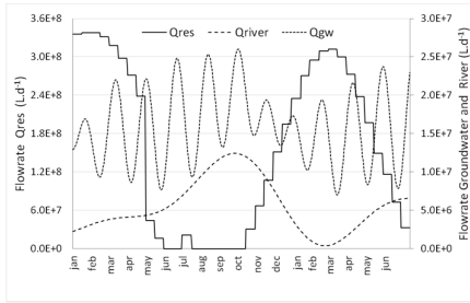
Figure 3. Inflow profiles into Chasicó Lake from the river ( Q_{river} ), groundwater ( Q_{GW} ) and reservoir ( Q_{res} ), for a 555-day dry period
