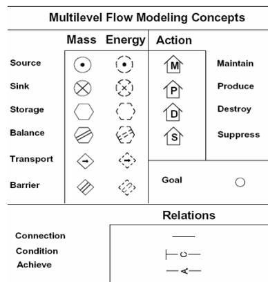
Fig.1. Multilevel flow modeling concepts
