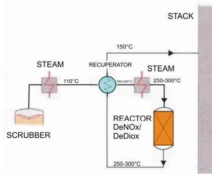
Fig.2 Scheme of DeNO<sub>x</sub>/DeDiox technology
