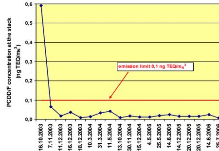
Fig.4 Result of PCDD/F measurements
