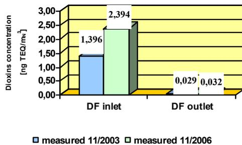
Fig.3 Efficiency of dioxin destruction in DF
