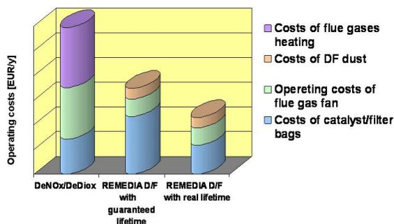
All running cost linked with a one year operation of the unit is included. The operating cost of the catalytic filtration DeNOx/DeDiox rises due to the reheating of flue gases to the required temperature of the reaction of about  $250 \text{ }^\circ\text{C}$  and the cost linked with the increased pressure drop (Fig.5).
