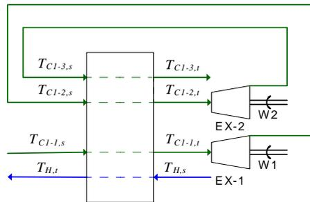
Figure 1 System with heat exchanges and expanders
