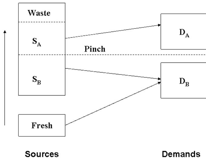
Fig.1. The illustration of the allocation of the source streams to the demand streams
