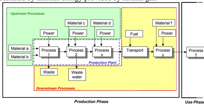
Fig. 2 Example schema of LCA boundary
