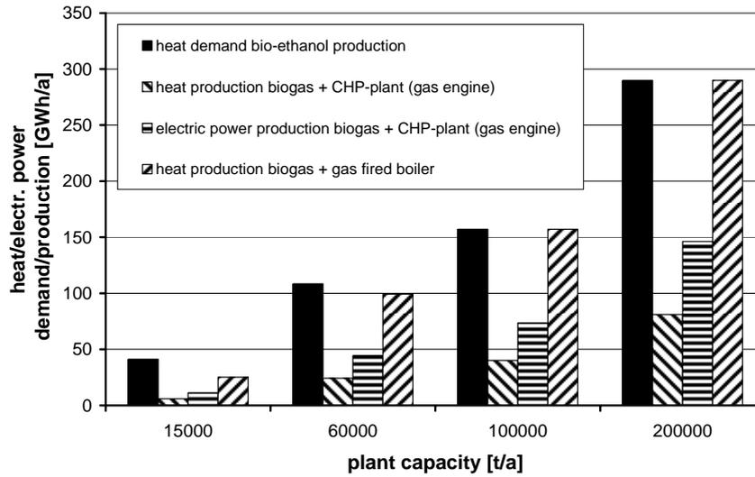
Figure 3: Heat demand during bio-ethanol production from wheat and generation of heat and electric power from biogas in CHP-plant (gas engine) and gas fired boiler
