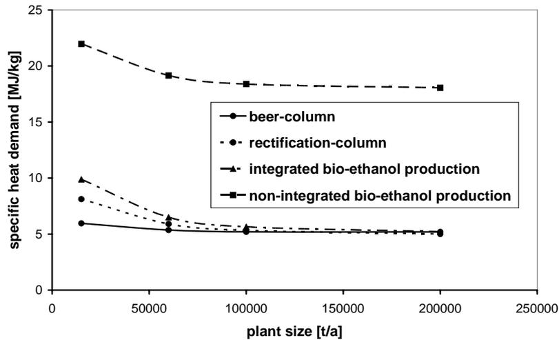
Figure 2: Specific heat demand of single units as well non-integrated and integrated bio-ethanol production facility for feedstock wheat
