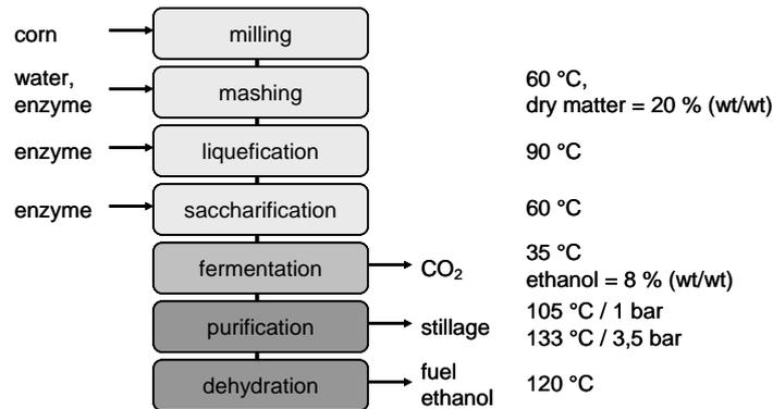
Figure 1: Scheme of bio-ethanol process
