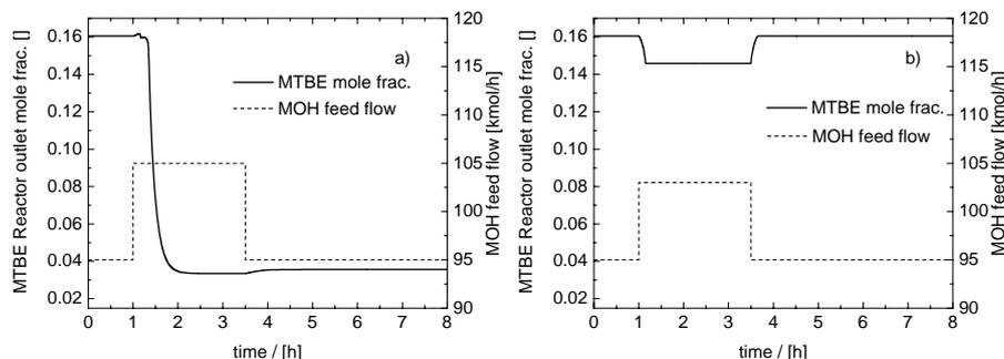
Figure 4. Comparison of evolution diagrams of a failure of MOH flow rate for 2.5 hours duration. a) step change to  $105 \text{ kmol}\cdot\text{h}^{-1}$  b) step change to  $103 \text{ kmol}\cdot\text{h}^{-1}$
