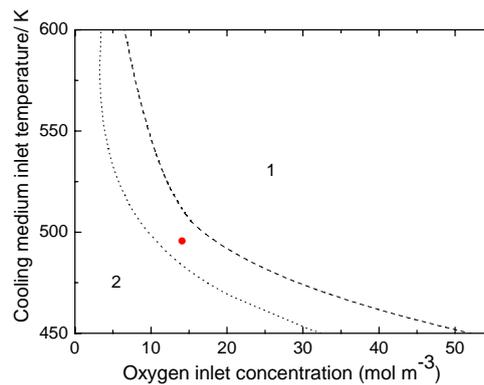
Figure 2. Locus of the run-away effect for the plot cooling medium temperature vs. oxygen inlet concentration circle corresponds to the normal reactor operation point, dashed line limits the region of the possible reactor run-away
