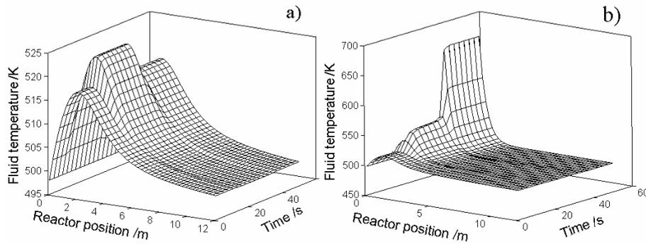
Figure 1. Dynamic evolution of the temperature profile along the reactor for different positive deviations from the input oxygen molar flow rate: a) 20 %, b) 23
