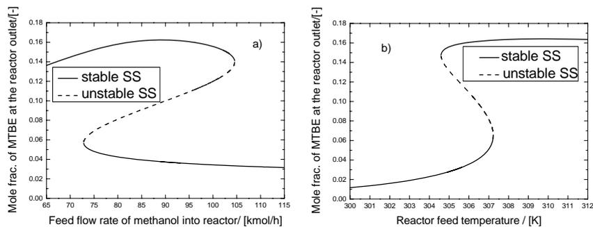
Figure 3. Solutions diagrams for the continuation parameter a) Feed flow rate of methanol into the reactor b) Reactor feed temperature
