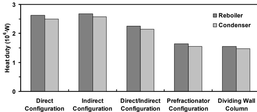
Figure 3. Reboiler and condenser heat duties for different distillation sequences
