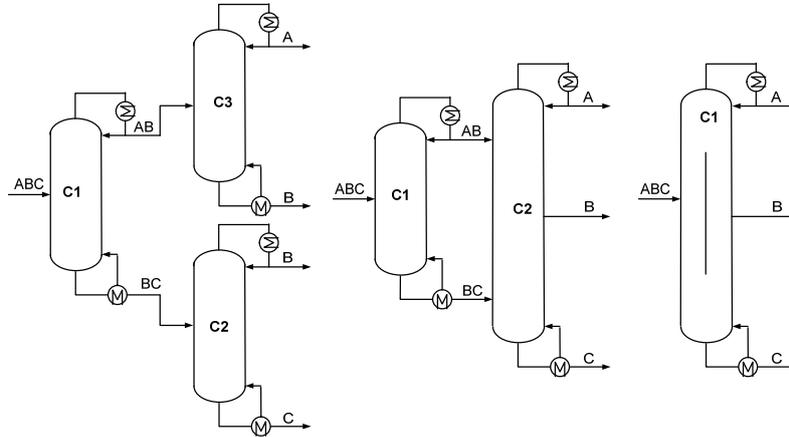
Figure 2. Simple column arrangement for separation of ternary mixtures: direct/indirect sequence (left); prefractionator configuration (centre); dividing wall column (right)
