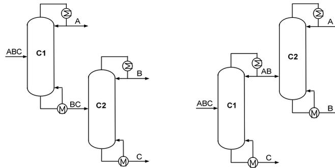
Figure 1. Conventional column arrangements for separation of ternary mixtures: direct sequence (left); indirect sequence (right)
