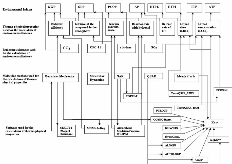
Fig. 1 Molecular modelling software used for the calculation of impact categories
