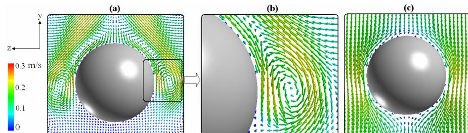
Fig. 5. Vector plot of liquid velocity field around single particle. Here the inlet air velocity is 0.5 and 0.01 m/s for parts a and c respectively. To obtain better visualization of flow field around the particle, the flow patterns marked in (a) is magnified and represented in (b).
