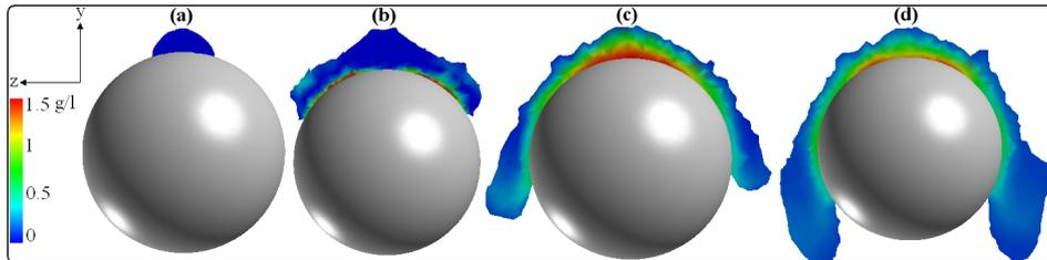
Fig. 2. Snapshots of the concentration profile of ferric ion. Realizations each separated by 0.01 s and the simulation was carried out for the inlet air velocity of 0.01 m/s.
