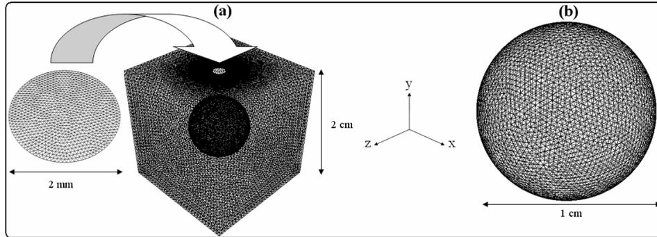
Fig. 1. (a) grid and dimensions of the computational domain and liquid entrance, (b) particle grid.
