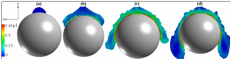
Fig. 3. Snapshots of the concentration profile of zinc ion on the surface of particle. Realizations each separated by 0.01 s and the simulation was carried out for the inlet air velocity of 0.01 m/s.
