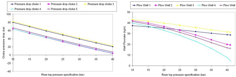
Figure 4: INDISS-TINA results from various riser top pressure specifications
