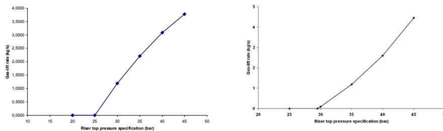
Figure 3: Cases with recycle – FP strategy Results from various riser top pressure specifications
