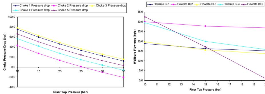
Figure 2.: Results from various riser top pressure specifications
