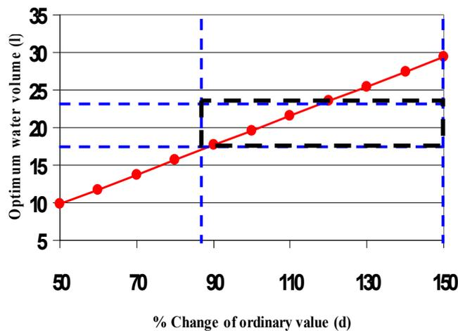
Figure 2 Optimal volume of rinse water with respect to drag-out volume change
