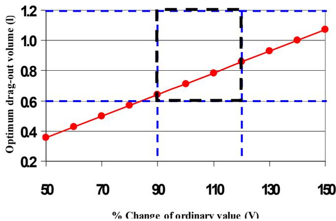
Figure 3 Optimal volume of drag-out with respect to water volume change
