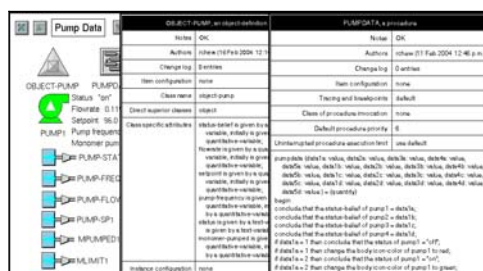
Figure 4. A workspace showing a pump definition.
