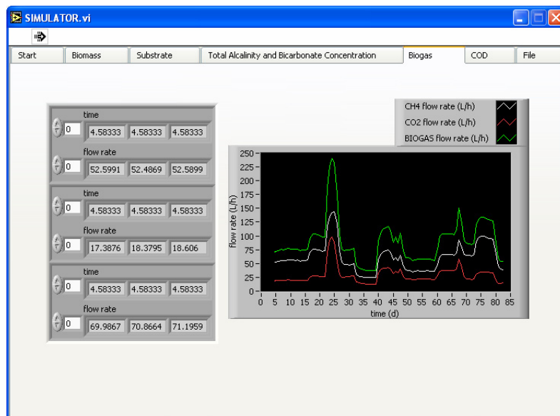
Figure 3. IRIN for dynamic simulation of the anaerobic digester in a wastewater treatment plant developed using LabVIEW®. Model and data adapted from Bernard et al., 2001.
