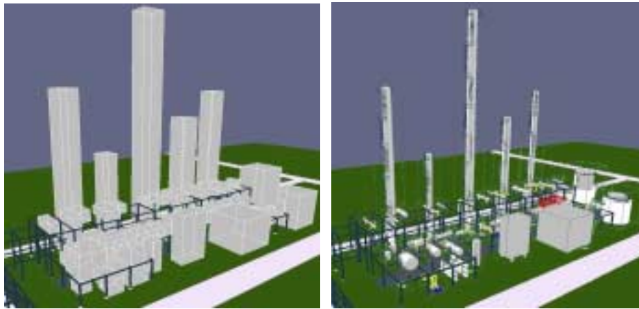
Fig. 3: Layout model represented by overall boxes and detailed equipment models
