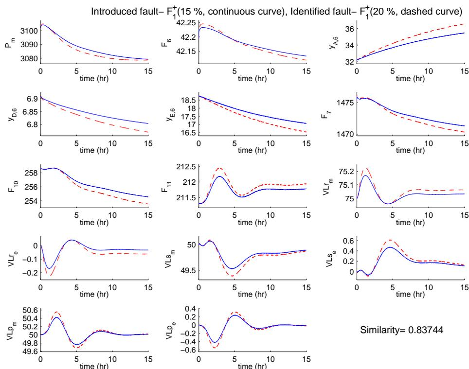
Figure 2: Sensor trends for simulated fault 1 and identified fault 1
