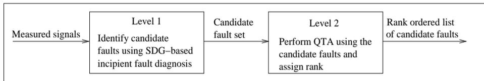
Figure 1: SDG-QTA based integrated framework for incipient FD
