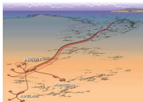
Figure 3 : Overview of offshore Snøhvit field with pipelines and onshore LNG plant in background.
