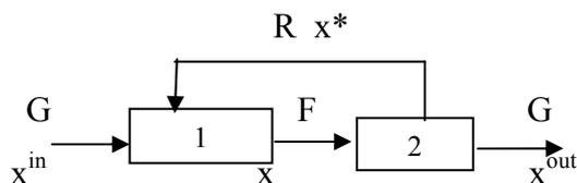
Figure 1. Reactor-separator recycle system: (1)-reactor, (2) - distillation column.
