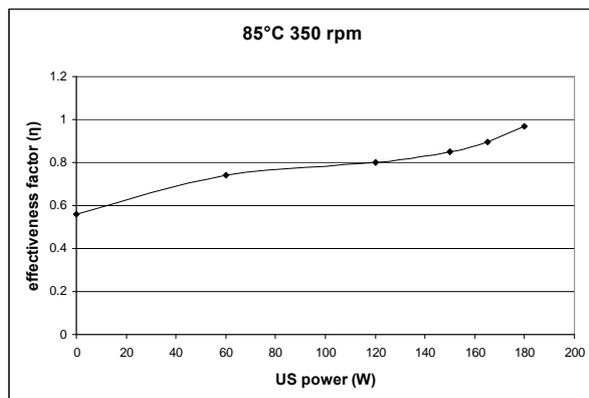
Figure 3. The effectiveness factor as a function of the induced ultrasonic power. Experiments were performed at 85°C with an agitation rate of 350 rpm.
