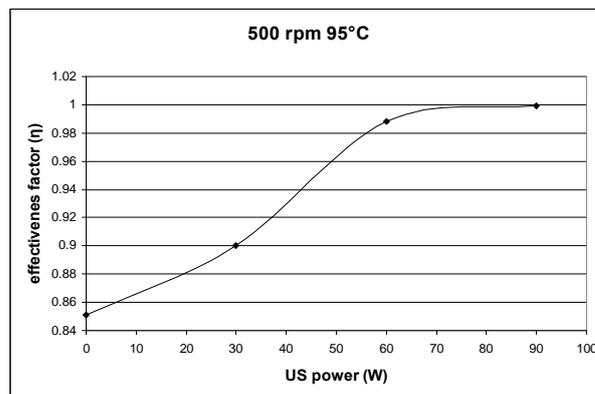
Figure 4. The effectiveness factor as a function of the induced ultrasonic power. Experiments were performed at 95°C with an agitation rate of 500 rpm.
