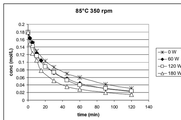
Figure 2. The concentration of ferric iron as a function of time for experiments performed with different ultrasonic power. Experiments were performed at 85°C with an agitation rate of 350 rpm.
