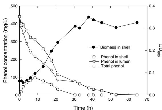
**Fig. 3.** Cell growth and phenol degradation in hollow fibers in the presence of 7.5 wt% NaCl in the lumen
