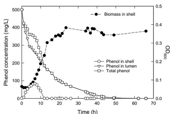
**Fig. 2.** Cell growth and phenol degradation in hollow fibers in the presence of 5 wt% NaCl in the lumen
