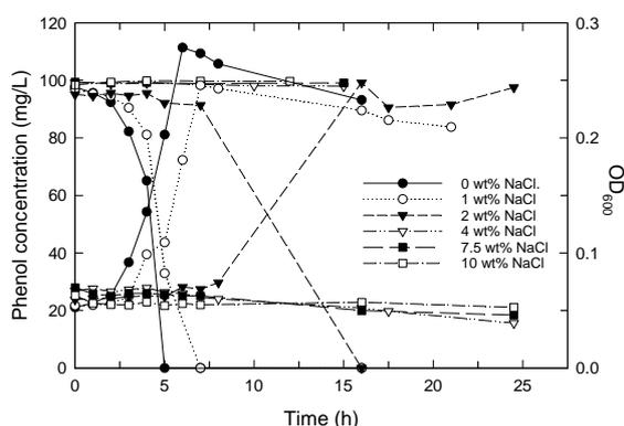
**Fig. 1.** Effect of added NaCl level on cell growth and degradation of phenol by suspended cells (pH 6.8)
