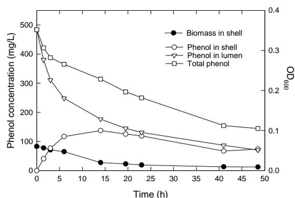
**Fig. 4.** Cell growth and phenol degradation in hollow fibers in the presence of 10 wt% NaCl in the lumen
