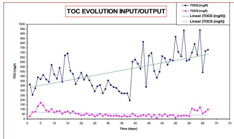
**Figure 2:** TOC evolution input/output in reactor
