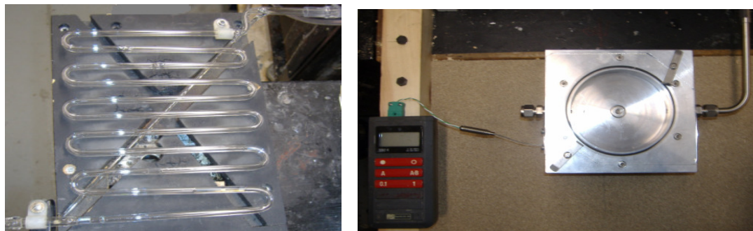
Figure 1 the narrow channel glass reactor (left) and the static film cell (right).
