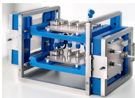
Figure 1: An example of a Corning Glass Micro Reactor
