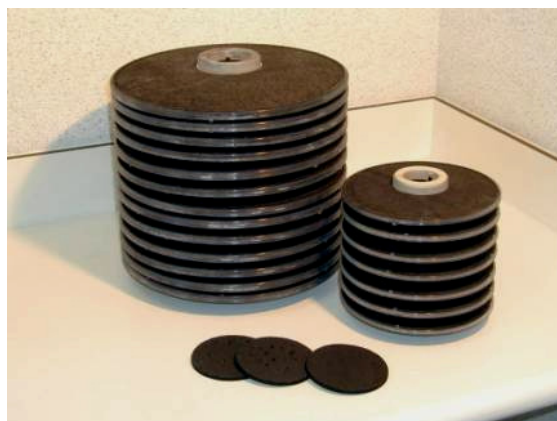
Figure 1: Example of CUNO ZetaCarbon discs for three different scale filters (~80 ml, ~ 32 l, ~ 300 l)
