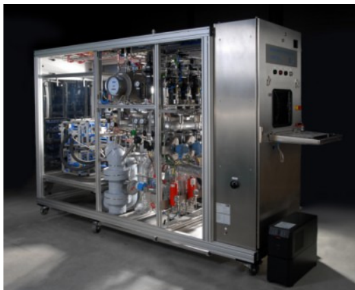
Figure 3: The industrial mobile multi-purpose micro reactor unit
