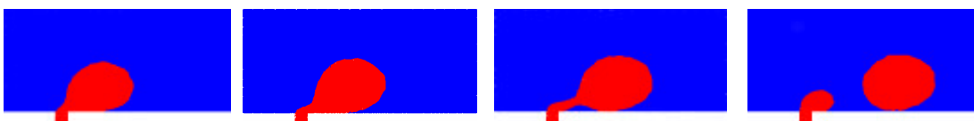
Figure 3. Droplet formation in the symmetry plane as calculated using 3D CFD simulations (VOF method).
