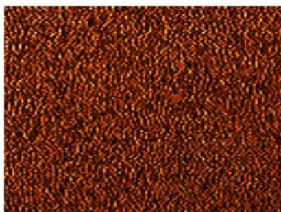
Figure1- plan view AFM micrograph of a 4nm thin Au film on Si before annealing
