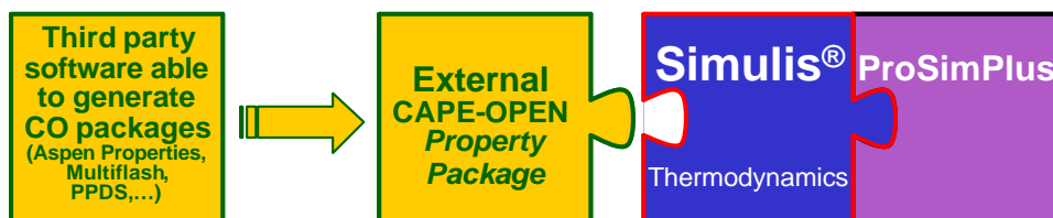
Figure 1: CAPE-OPEN thermodynamic socket
