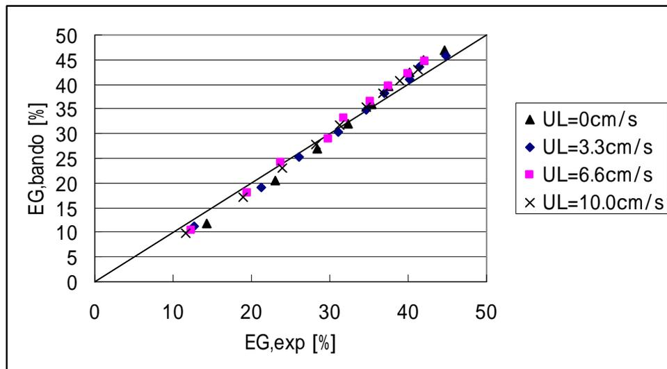
Fig.8 Comparison between  $E_{G,exp}$  and  $E_{G,Bando}$  calculated from Eqs.(6) and (7) for  $H_{in} = 0$  cm.
