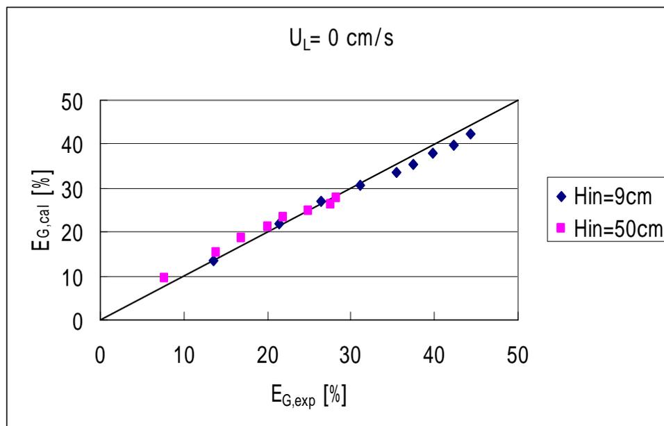
Fig.3  $E_{G,cal}$  vs.  $E_{G,exp}$  at  $U_L = 0$  cm/s.
