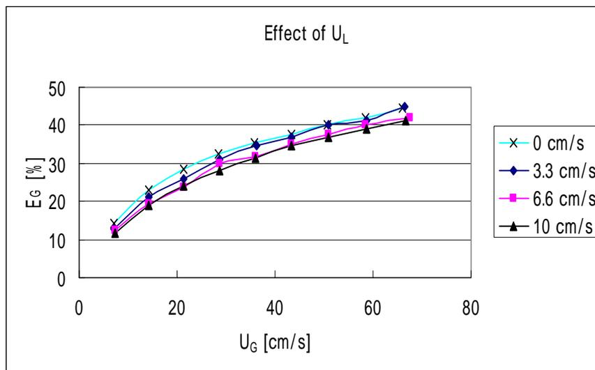
Fig.5 Effect of  $U_L$  on  $E_G$  at  $H_{in} = 0$  cm.
