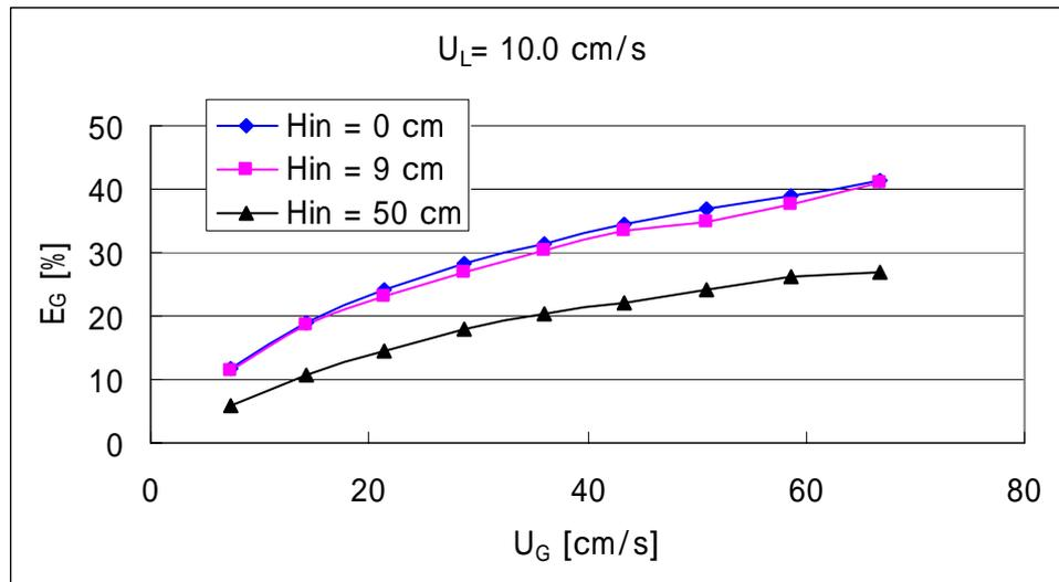
Fig.2 Effect of  $H_{in}$  on  $E_G$  at  $U_L = 10.0$  cm/s.
