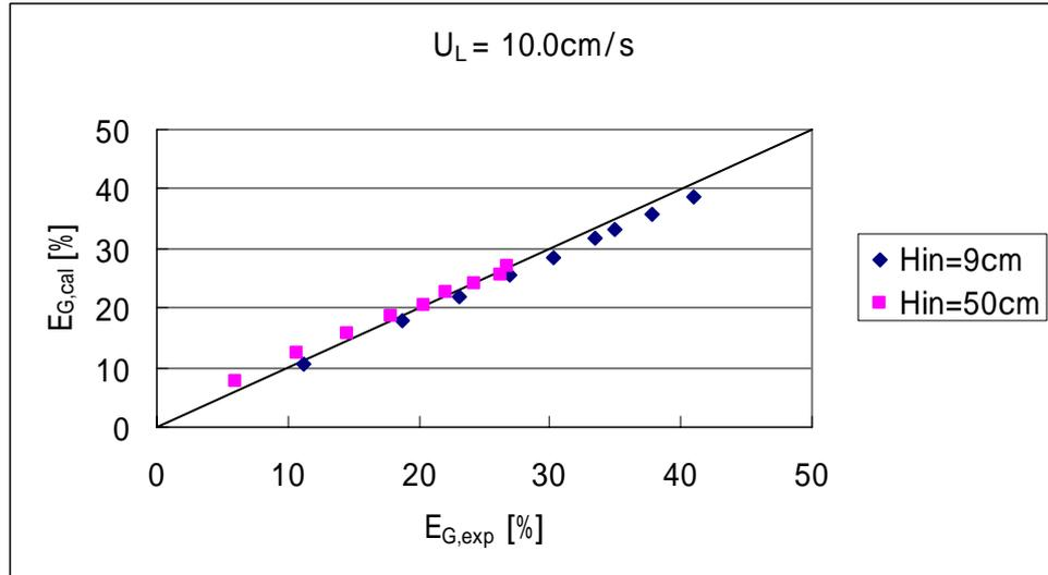
Fig. 4  $E_{G,cal}$  vs.  $E_{G,exp}$  at  $U_L = 10.0$  cm/s.
