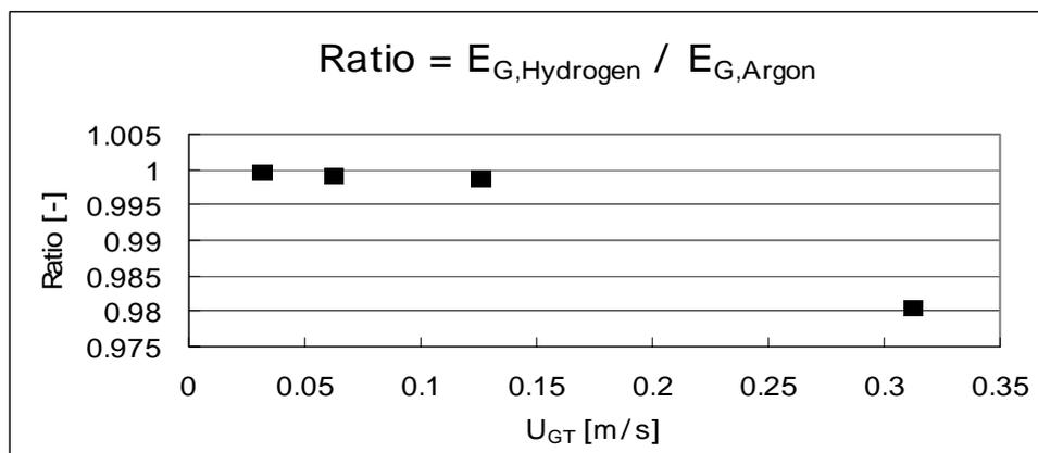
Fig.14 Effect of kinds of gas on  $E_G$  by the simulation
