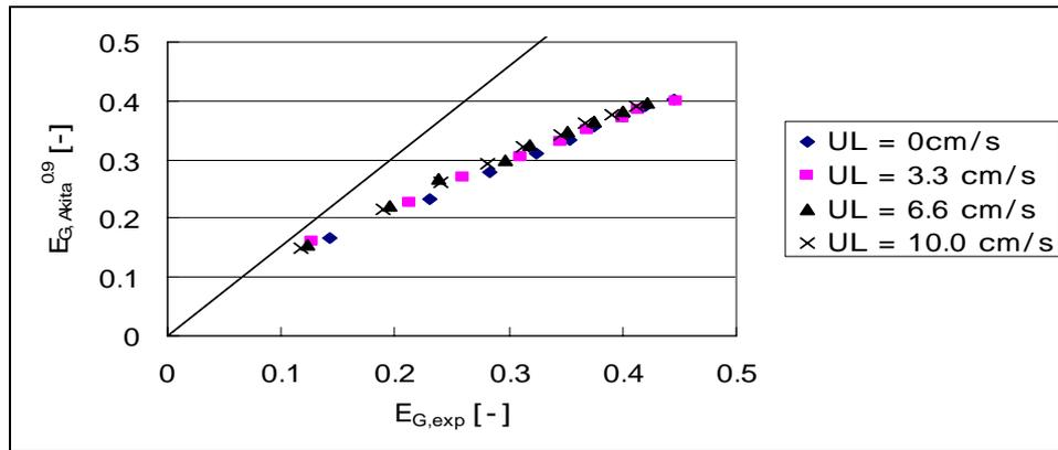
Fig.7 Comparison between  $E_{G,exp}$  and  $E_{G,Akita}^{0.9}$  from Eq.(2) for  $H_{in} = 0$  cm.
