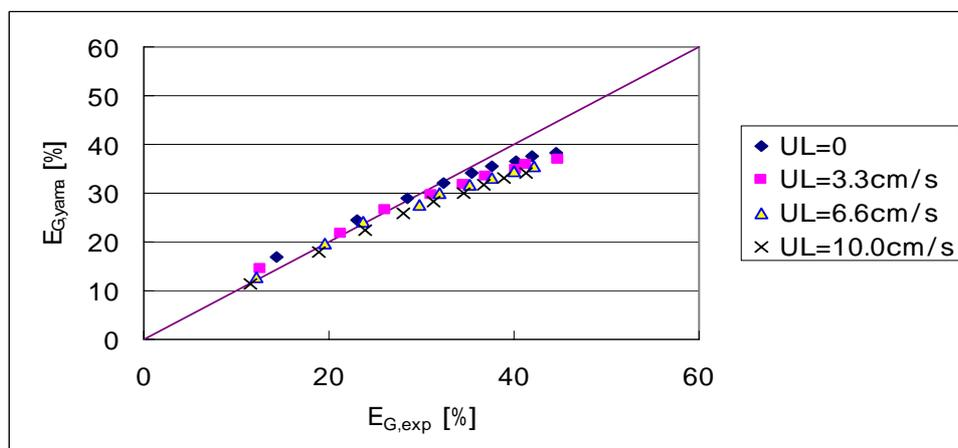
Fig.9 Comparison between  $E_{G,exp}$  and  $E_{G,yama}$  calculated from Eq.(9) for  $H_{in} = 0$  cm.
