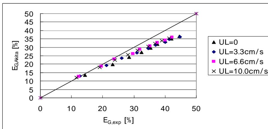
Fig.6 Comparison between  $E_{G,exp}$  and  $E_{G, Akita}$  by Eq.(2) for  $H_{in} = 0$  cm.
