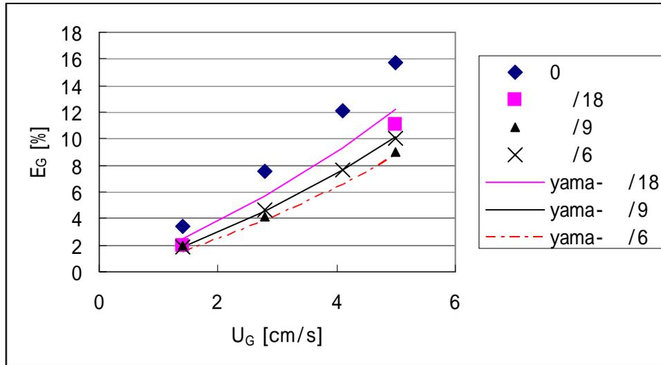
Fig.16 Effect of column inclination on  $E_G$ .
