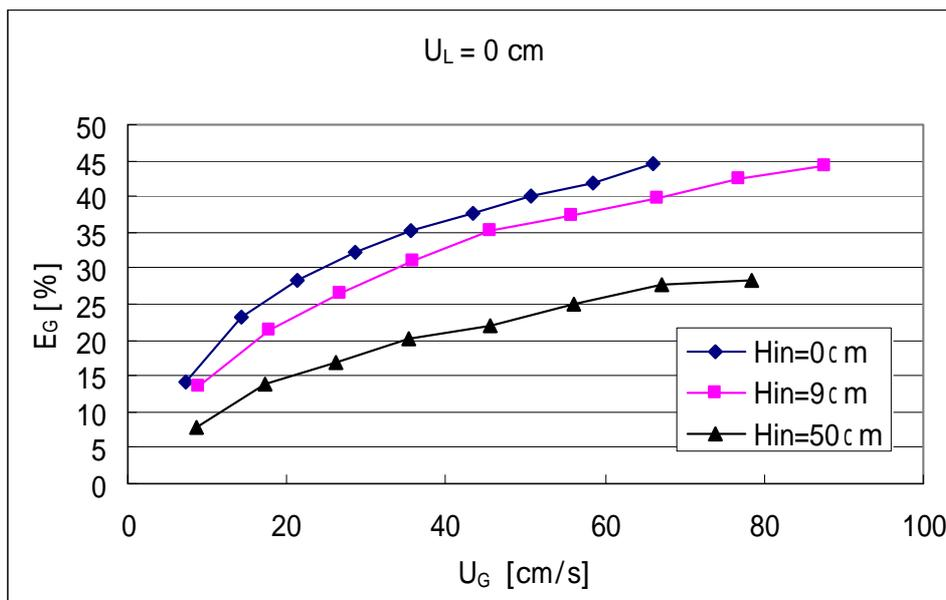
Fig.1 Effect of  $H_{in}$  on  $E_G$  at  $U_L = 0$  cm/s.
