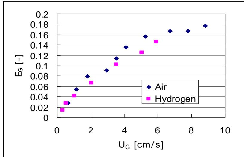
Fig.10 Effect of kinds of gas on  $E_G$  in the No.2 bubble column.
