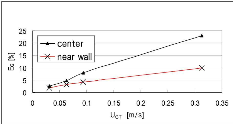
Fig.15 Effect of arrangement of gas inlet on  $E_G$
