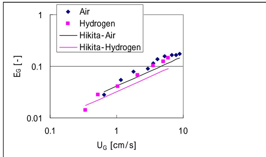
Fig.11 Comparison between the correlation by Hikita et al.(1980) and  $E_G$  in the No.2 bubble column.
