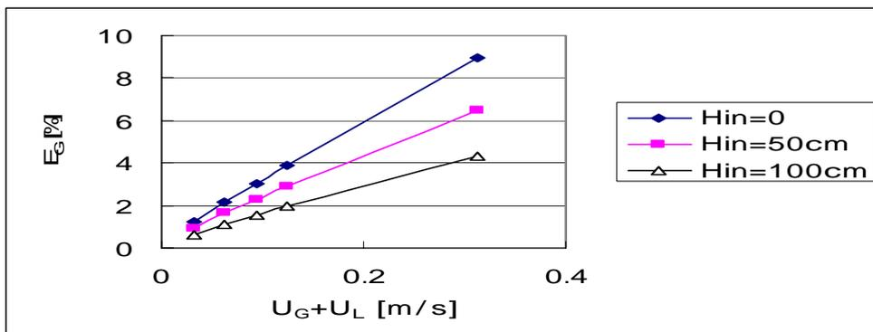
Fig.12 Effect of gas inlet height  $H_{in}$  on  $E_G$ .
