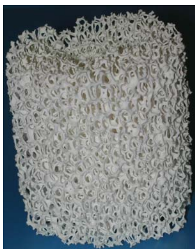
Fig. 1. (a) Real and (b) modeled structure of a highly porous cellular material.
