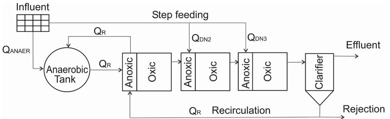
Figure 2. Experimental set-up of the BNRAS system.
