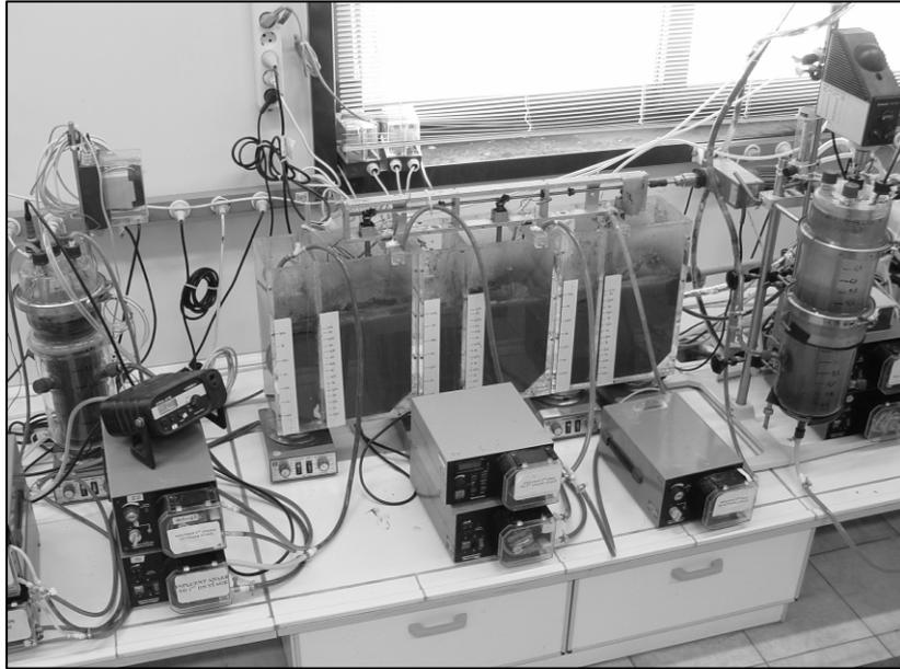
**Figure 1. View of the Biological Nutrient Removal Activated Sludge (BNRAS) system.**
