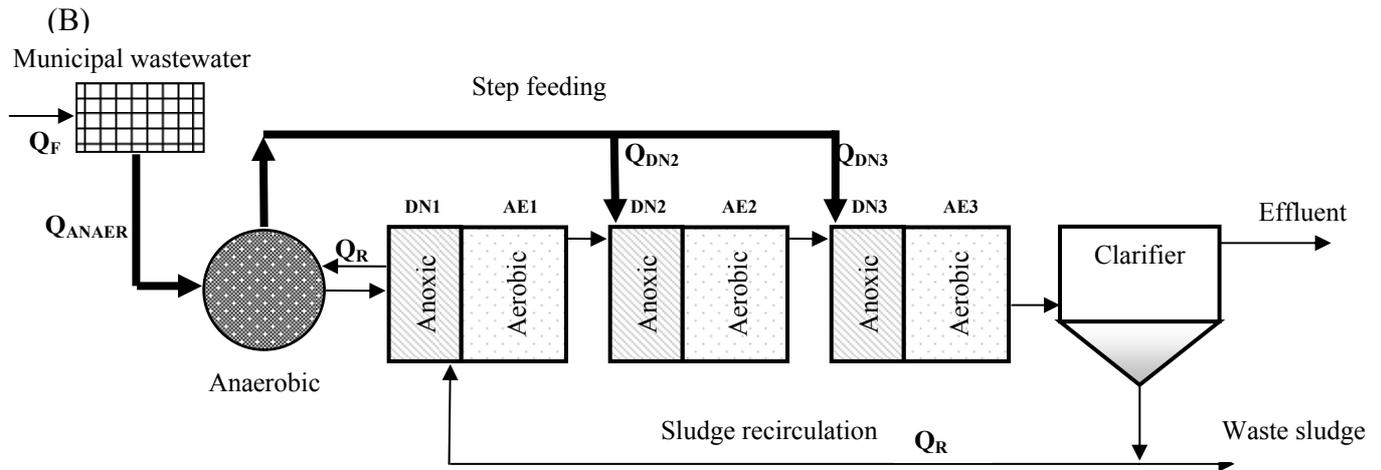
**Figure 3. Schematic layout of the feed distribution pattern (A) before and (B) after the anaerobic selector in the pilot scale BNRAS plant.**
