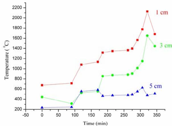
Figure 3: Classical temperature profile at distances of 1, 3 and 5 cm from the heater axes
