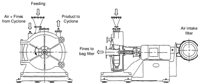
Figure 2.2.1 - Frontal and side view of a Donaldson Acucut<sup>®</sup> Air Classifier – Hosokawa Micron Inc.
