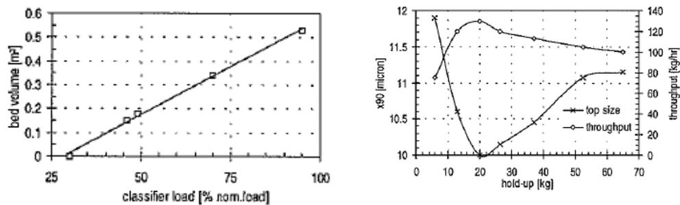
Figure 5.1 - Power draw of the ATP classifier motor as an indirect measure of circulation load (left) and correlation between hold-up and particle size (Gommeren, 1997)
