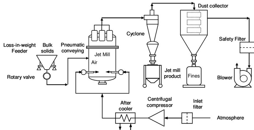
Fig 2.2 - General arrangement of the grinding plant.
