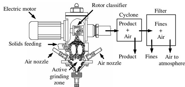
Figure 2.1 - The Fluidized Bed Opposed Jet Mill AFG-100.
