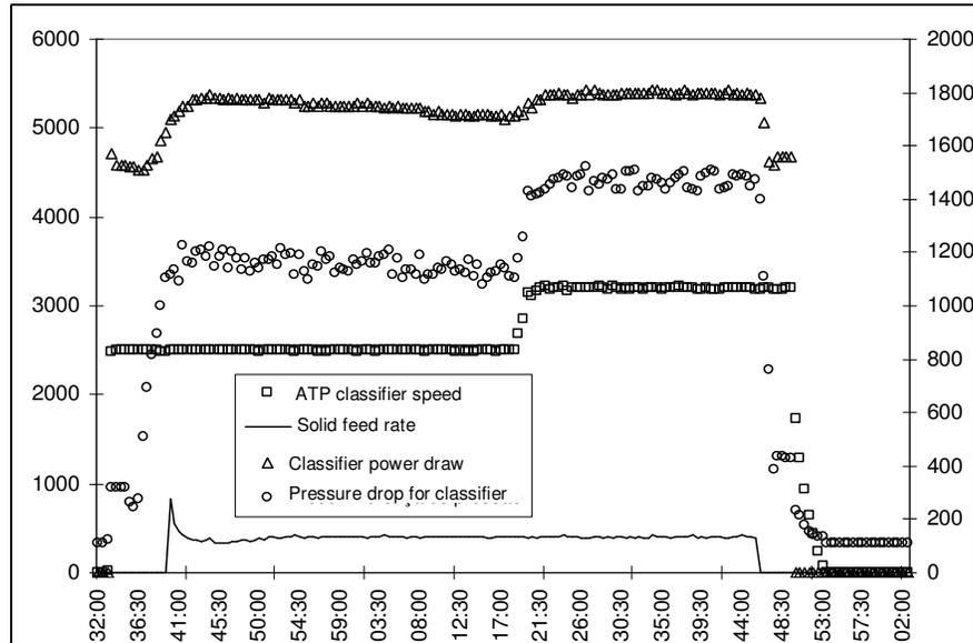
Figure 5.2 - Pressure drop for the classifier and power draw in the ATP classifier motor
