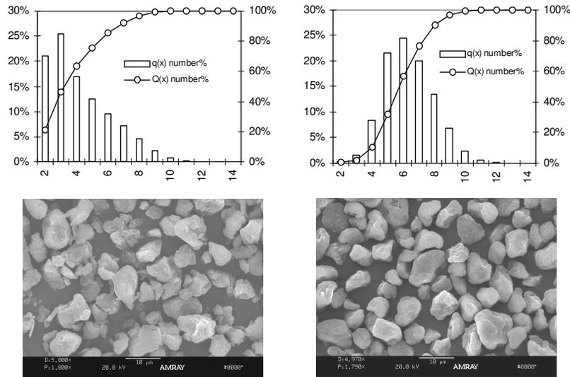
Figure 3.1.1.1 – Size distribution and of the material after the grinding process (left) and after air classification (right).
