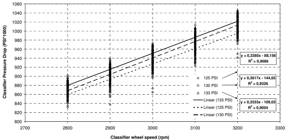
suggests the possible use of pressure transmitter readings as a virtual on line sensor for particle size. An additional experiment was used to evaluate the influence of rotor speed and
