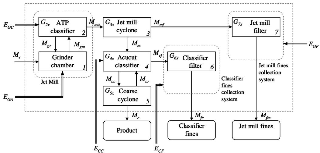
Figure 3.3.2.1 – Energy efficiency of the extended size reduction plant.
