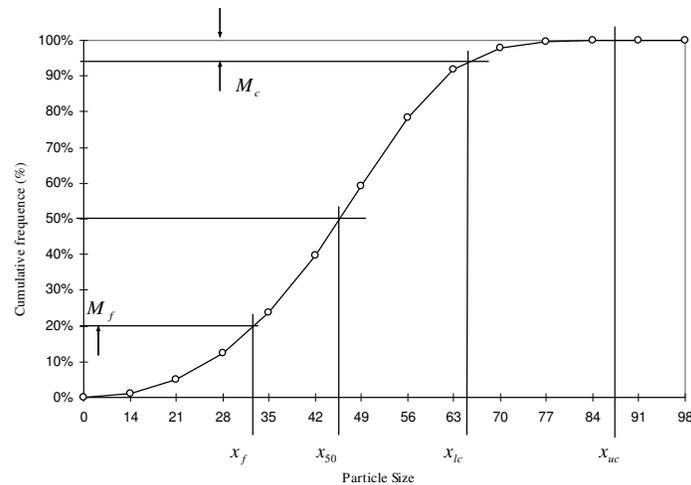
Figure 3.1.1.2 - Cumulative frequency distribution - PSD parameters used to express product quality.
