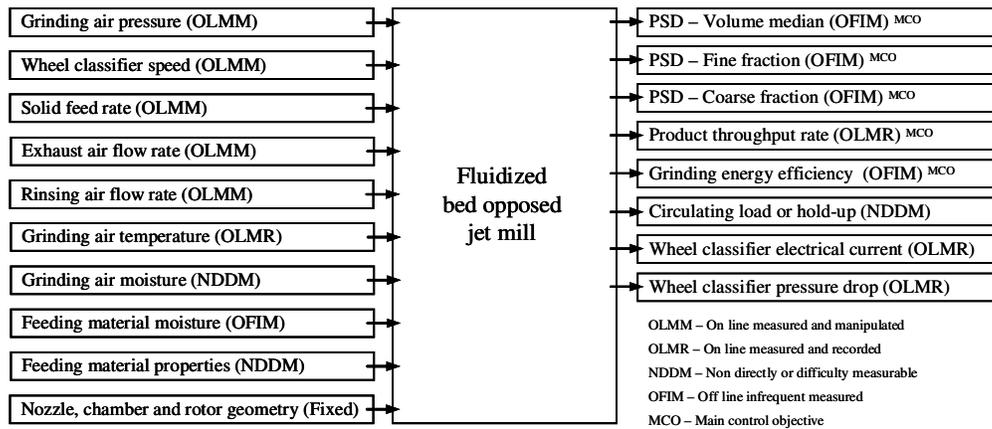
Figure 3.1.1 - The fluidized opposed jet mill as a black box: Inputs, outputs and available data acquisition.
