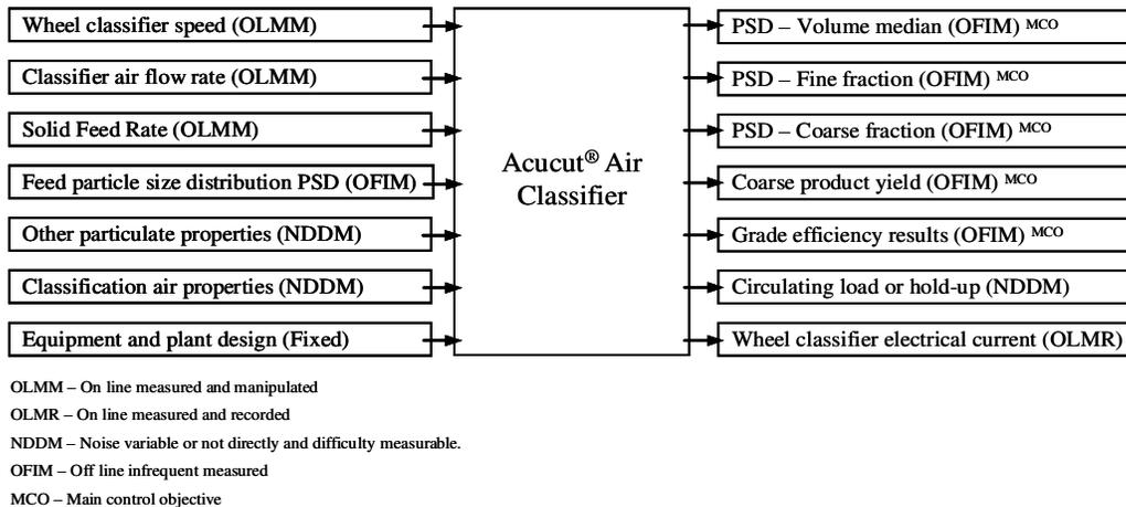
Figure 7 - The Acucut Air Classifier as a black box: Inputs, outputs and available data acquisition
