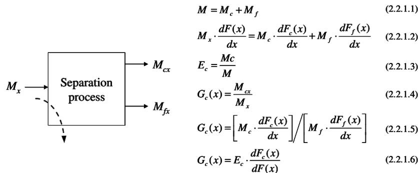
Figure 2.2.1.1 Grade efficiency method for a single separation process
