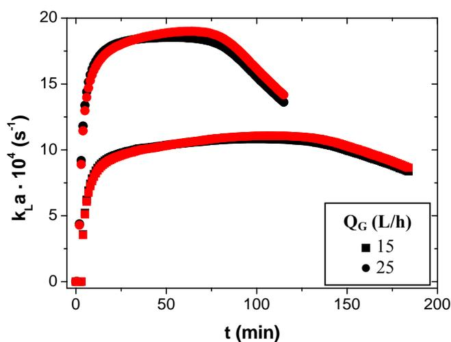
**Figure 5.** Temperature effect on volumetric mass transfer coefficient for a concentration of 0.3 M at different gas flow rate: constant temperature (black), variable temperature (red).
