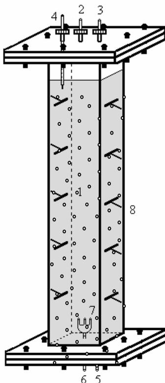
**Figure 1.** Schematic figure of the bubble column reactor: (1) Bubble column, (2) Liquid inlet, (3) Gas outlet, (4) Thermometer, (5) Liquid outlet, (6) Gas inlet, (7) Gas sparger, (8) Electrodes.
