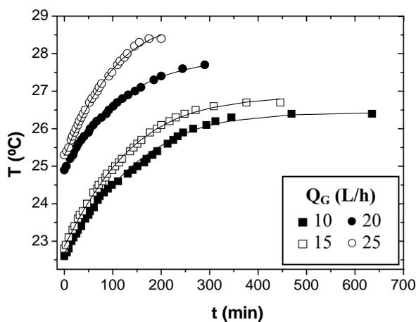
**Figure 2.** Temperature vs. time for a concentration of 1 M at different gas flow rate: (—) Boltzmann equation.
