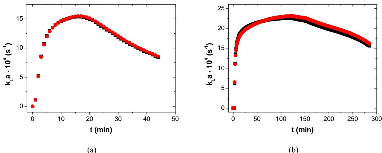
**Figure 4.** Temperature effect on volumetric mass transfer coefficient for a gas flow rate of 25 L/h and different MDEA concentrations: (a) 0.05 M and (b) 1.0 M; constant temperature (black), variable temperature (red).
