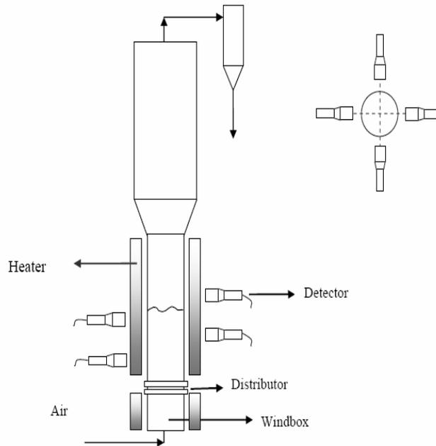
Figure 1. Schematic Illustration of Fluidized Bed Reactor
