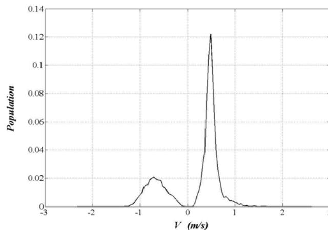
Figure 2. Velocity Distribution at Superficial Gas Velocity of 0.52 m/s and T=25 °C
