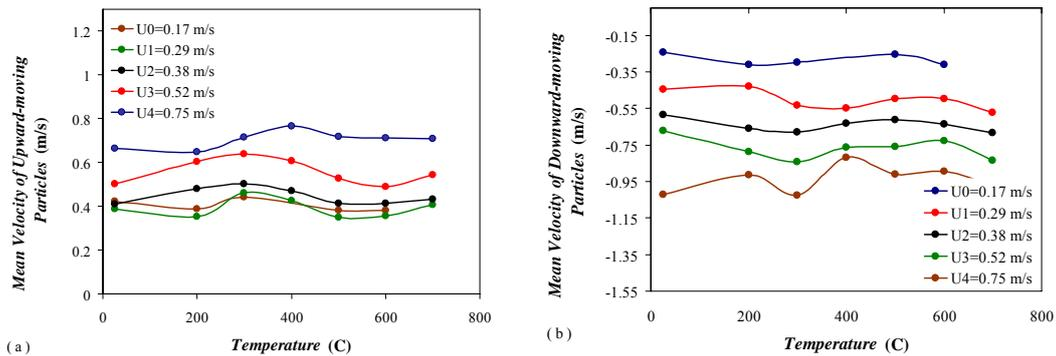
Figure 3. Mean velocity of particles as a function of temperature a) upward-moving b) downward-moving
