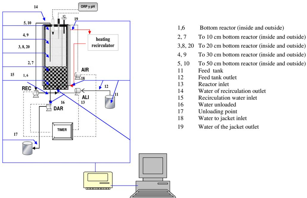
Figure 2. Diagram of the SBR anaerobic/aerobic for the treatment of the DR23.
