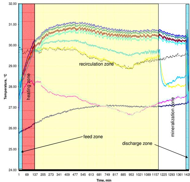
Figure 4. Temperature profiles for once cycle into the start up
