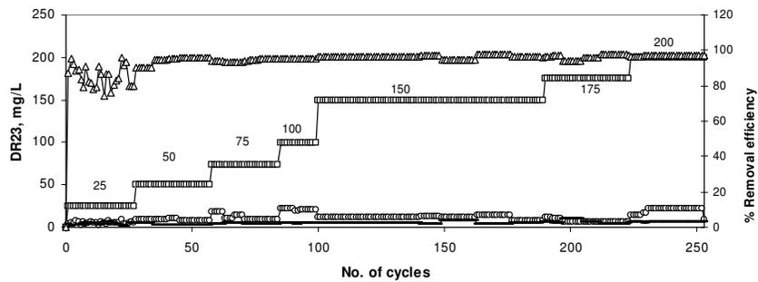
Figure 3. Performance of the SBR in the treatment of DR23. (■) Cycle start (●) Anaerobic phase end (-) Aerobic phase end (Δ) %Removal efficiency
