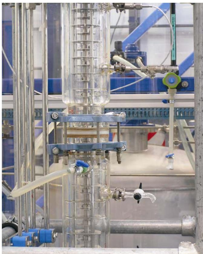
Figure 1. Pilot Rotating Disc Column
