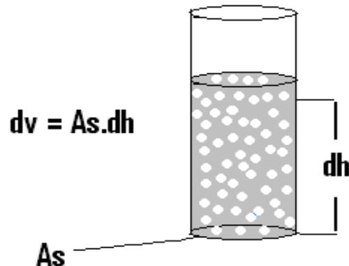
Figure 2 the control volume of oxygen in bubble column
