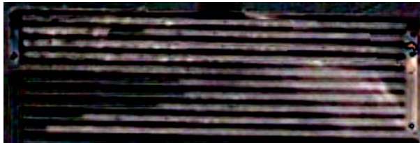
Figure 7: Liquid water in the serpentine design. Zoom in the upper part.
