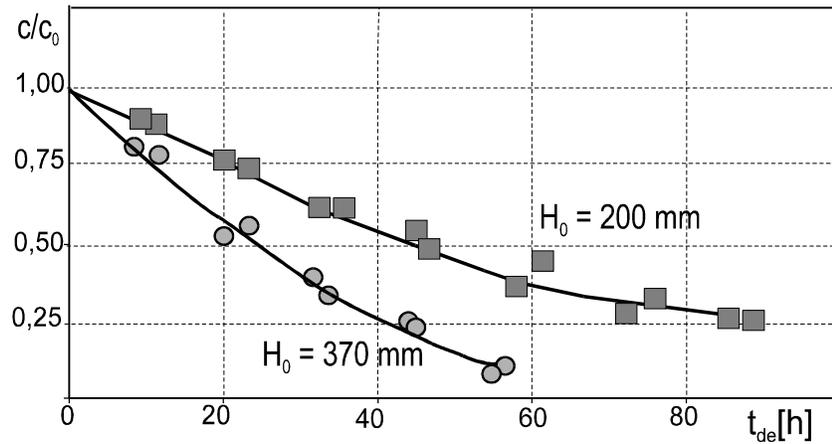
Fig. 3. Dimethylketone concentration changes during the degradation time in the inverse fluidized bed airlift reactor with immobilized bacteria for the gas velocity equal to the minimum fluidization velocity.  $c_{B0} = 0,4\%$  obj. pH = 7
