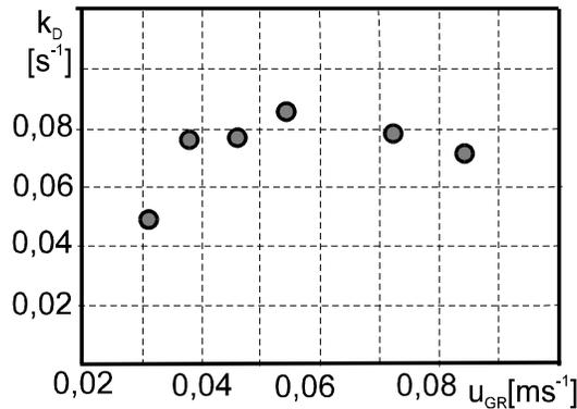
Fig. 4. Dependence of the degradation constant on the air flow rate. pH = 7,0;  $c_0 = 0,2 \%$  obj.,  $H_0 = 390$  mm
