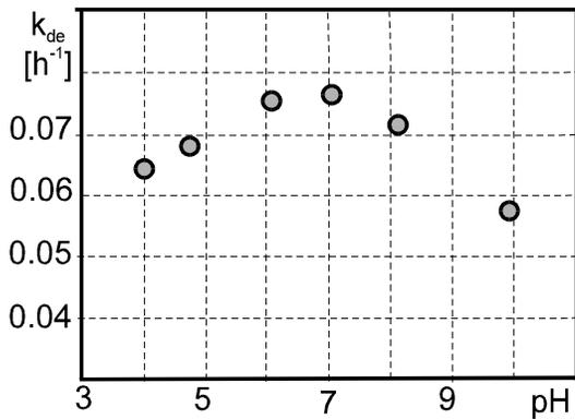
Fig. 2. Dependence of the degradation constant on the pH of aqueous dimethylketone solution.
