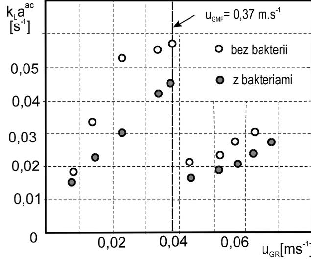
Fig. 5. Influence of the gas velocity on the oxygen accumulation rate in the fixed bed and in the inverse fluidized bed.  $d_s = 2,5$  mm.  $H_0 = 0,4$  m.  $pH = 7$
