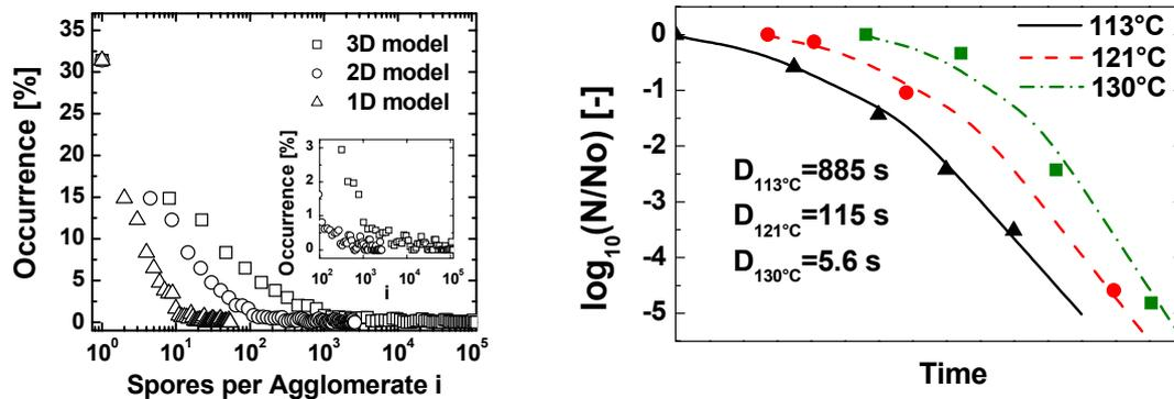
Fig. 3a): Agglomeration size distribution of a *G.stearothermophilus* spore suspension with different geometrical assumptions for the agglomerates and an inset, which shows agglomerations sizes between 10<sup>2</sup>-10<sup>5</sup> spores per agglomerate (Mathys, Heinz et al., 2007).
