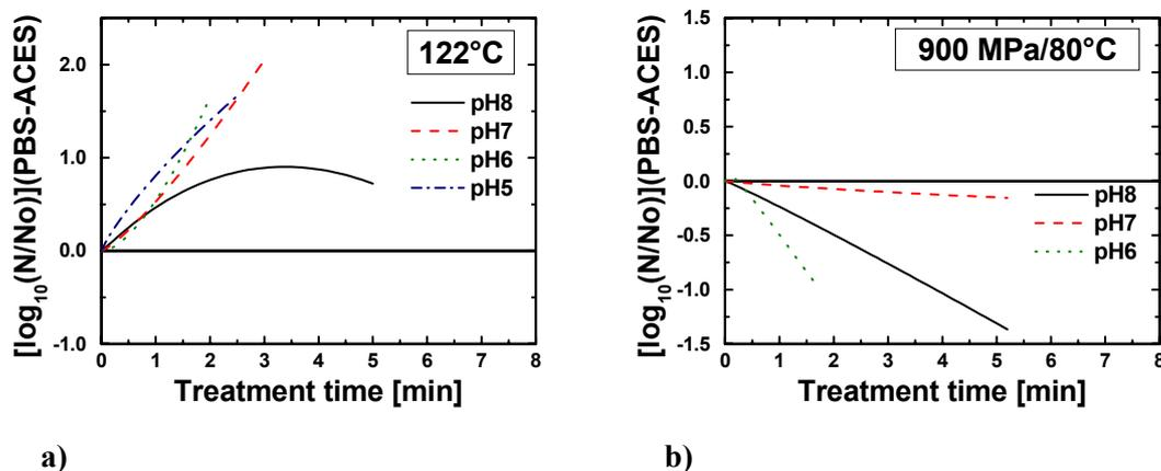
Fig. 1): Difference in  $\log_{10}$ -reduction of *G.stearotherophilus* spores in phosphate (PBS) and ACES ( $[\log_{10}(N/N_0)](\text{PBS-ACES})$ ) after thermal (122°C, Fig. 1a) and pressure (900 MPa at 80°C, Fig. 1b) treatment at different initial pH-values.
