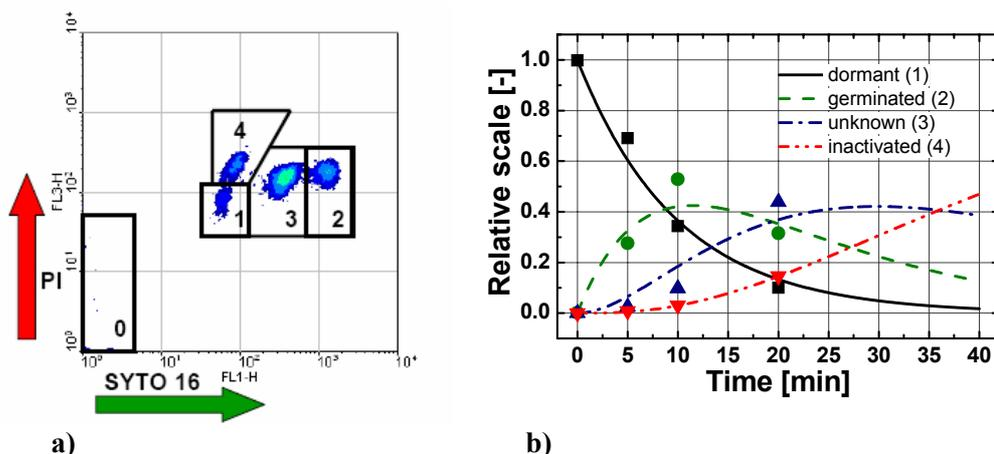
Fig. 2a): Sub-population assignment for density plot diagrams of *B.licheniformis* spores in sodium citrate buffer after treatment at 150 MPa with 37°C for 20 min: (0 = noise), 1 = dormant, 2 = germinated, 3 = unknown, 4 = inactivated (Mathys, Chapman et al., 2007).
