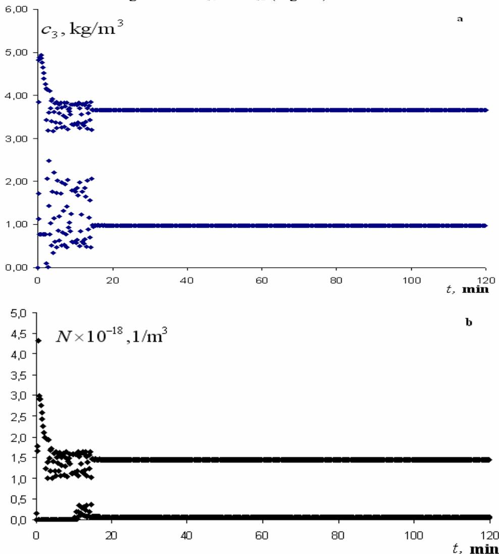
**Fig. 7.** Stabilization of the cycle of period-2 via proportional feedback method: the time dependences of (a) the concentration and (b) the number of clusters of dibasic lead phosphite ( $v_q = 13.26$  l/h) before and during the operation of control.
