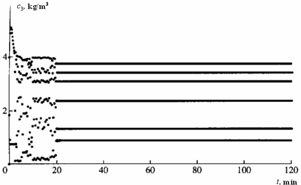
**Fig. 9.** Stabilization of the cycle of period-6 via destochastization method: the time dependences of the concentration of dibasic lead phosphite ( $v_q = 13.26$  l/h) before and during the operation of control.
