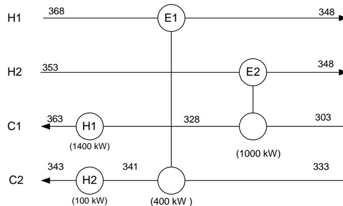
Figure 6 – Best HEN configuration with no stream splitting
