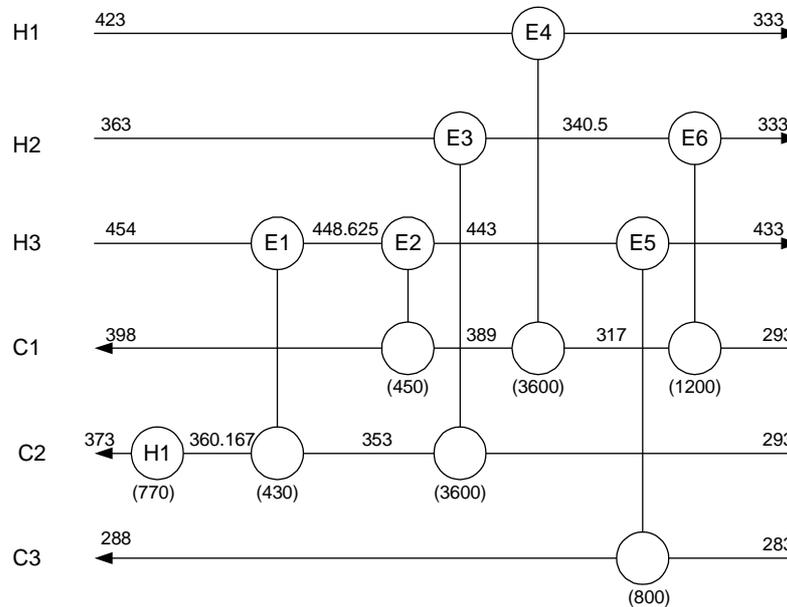
Figure 9 – Case 2 best HEN configuration with no stream splitting
