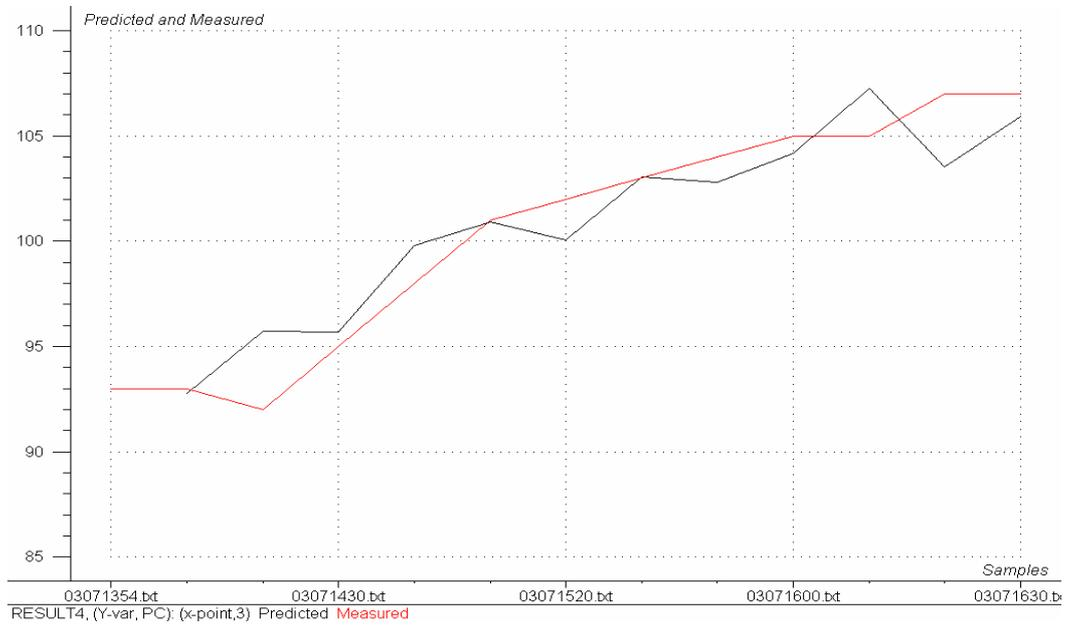
Figure 16. Predicted vs. measured UREA crystallisation-temperature in relation to the granulator experiment setting up an urea concentration gradient
