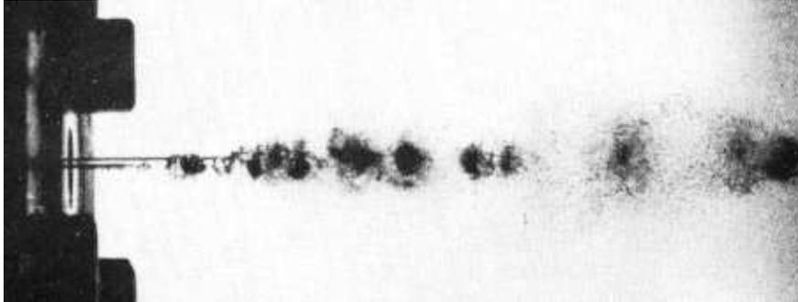
*Figure 1. Liquid flow through an orifice plate, note cavitations downstream generated by the relatively high pressure loss causing the local pressure to drop below the vapor pressure. (photo by Lienhard & Stephenson)*
