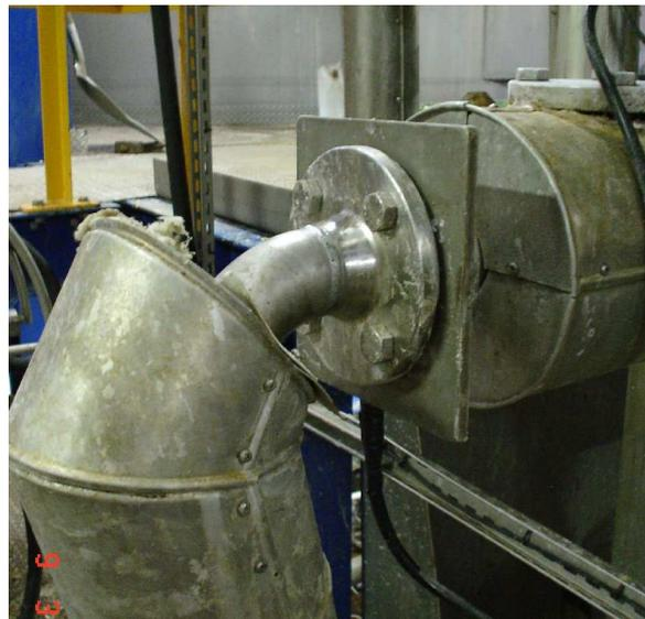
Figure 12. Acoustic sensor mounted on orifice plate in liquid feed line to granulator
