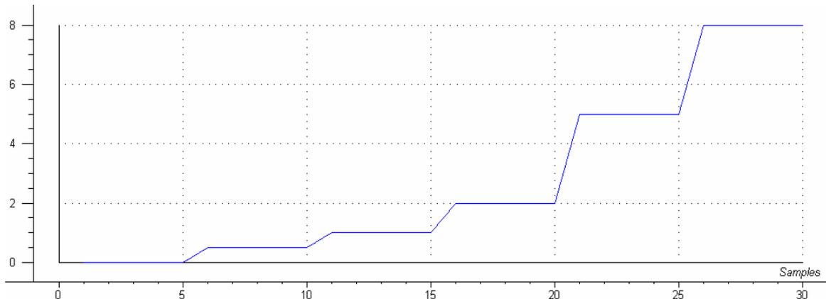
Figure 10 Ammonia concentration reference levels 0, 0.5, 1, 2, 5 and 8 % ammonia, 5 replicate measurements on each level.
