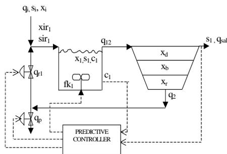
Figure 3: Plant and controller layout
