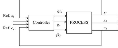
Figure 5: General controller structure
