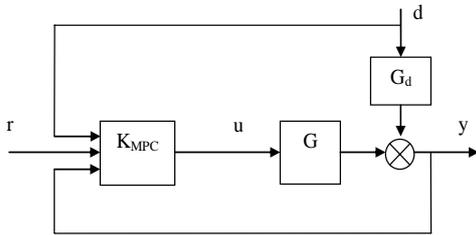
Figure 1 : Closed loop system with measured disturbances
