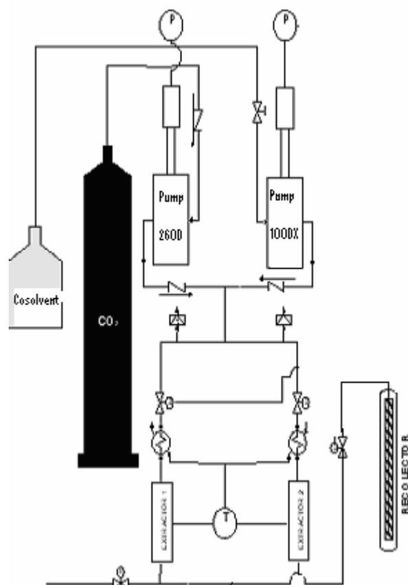
Figure 1. Schematic diagram of the analytical equipment.
