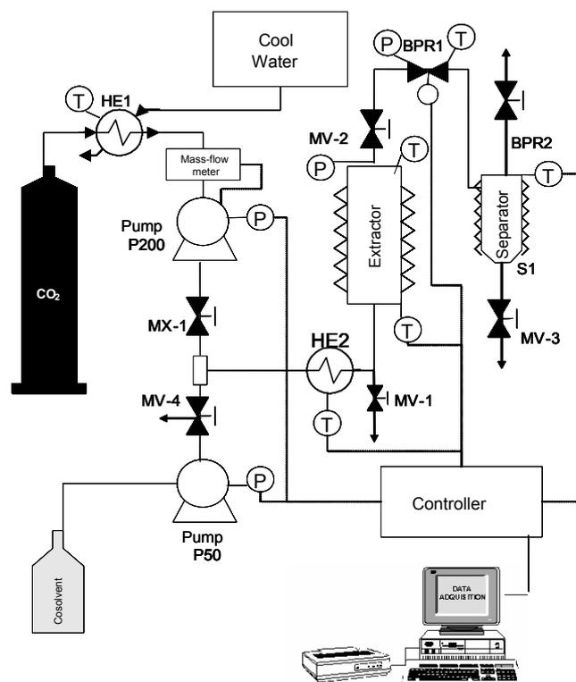
**Fig. 2.** Schematic diagram of the equipment used for the SFE.
