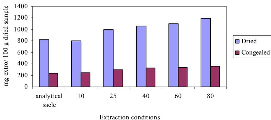
Fig 5. Comparison of the yields obtained in the extraction of bioactive substances with supercritical carbon dioxide on the two scales, to 50 °C, 400 bar and 300 minutes.
