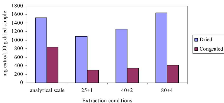
Fig 6. Comparison of the yields obtained in the extraction of bioactive substances with carbon dioxide and water on the two scales, to 50 °C, 400 bar and 300 minutes.
