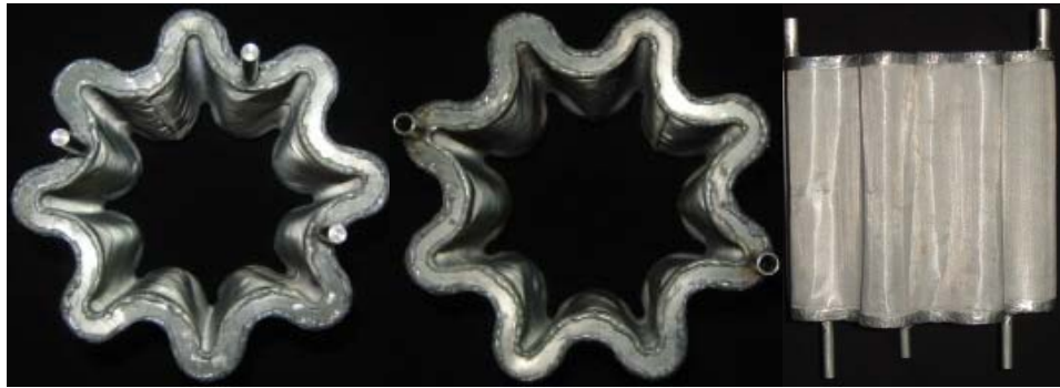
Fig. 1 Upper (a) and lower (b) cross view and axial view (c) of the design filtration module.
